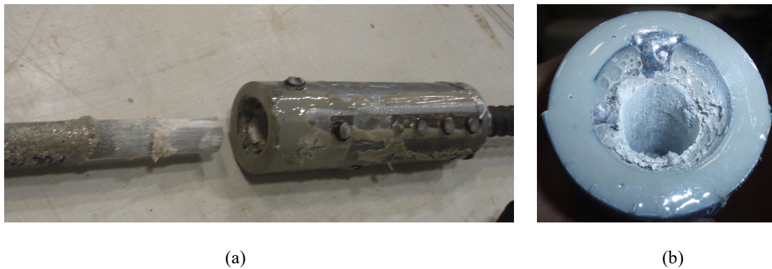
Fig. 17. Sand coated FRP bar connected to SBC with flattened screws and epoxy adhesives (a) failure pattern of FRP bar, and (b) inner face of epoxy adhesive inside coupler after pullout of FRP bar.
